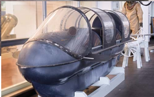
The HAVAS Mk IV manned submersible, an underwater vehicle for combat divers. (Photo: Forum Marinum, Jorma Kontio)
