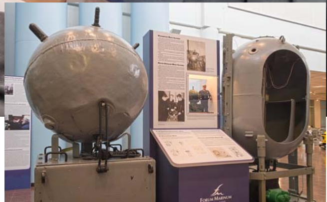
The contact mines S/40-A and S/36, and a statuette of an early Finnish Navy mine expert, Master Specialist Mikko Aaltonen. (Photo: Forum Marinum, Jorma Kontio)
