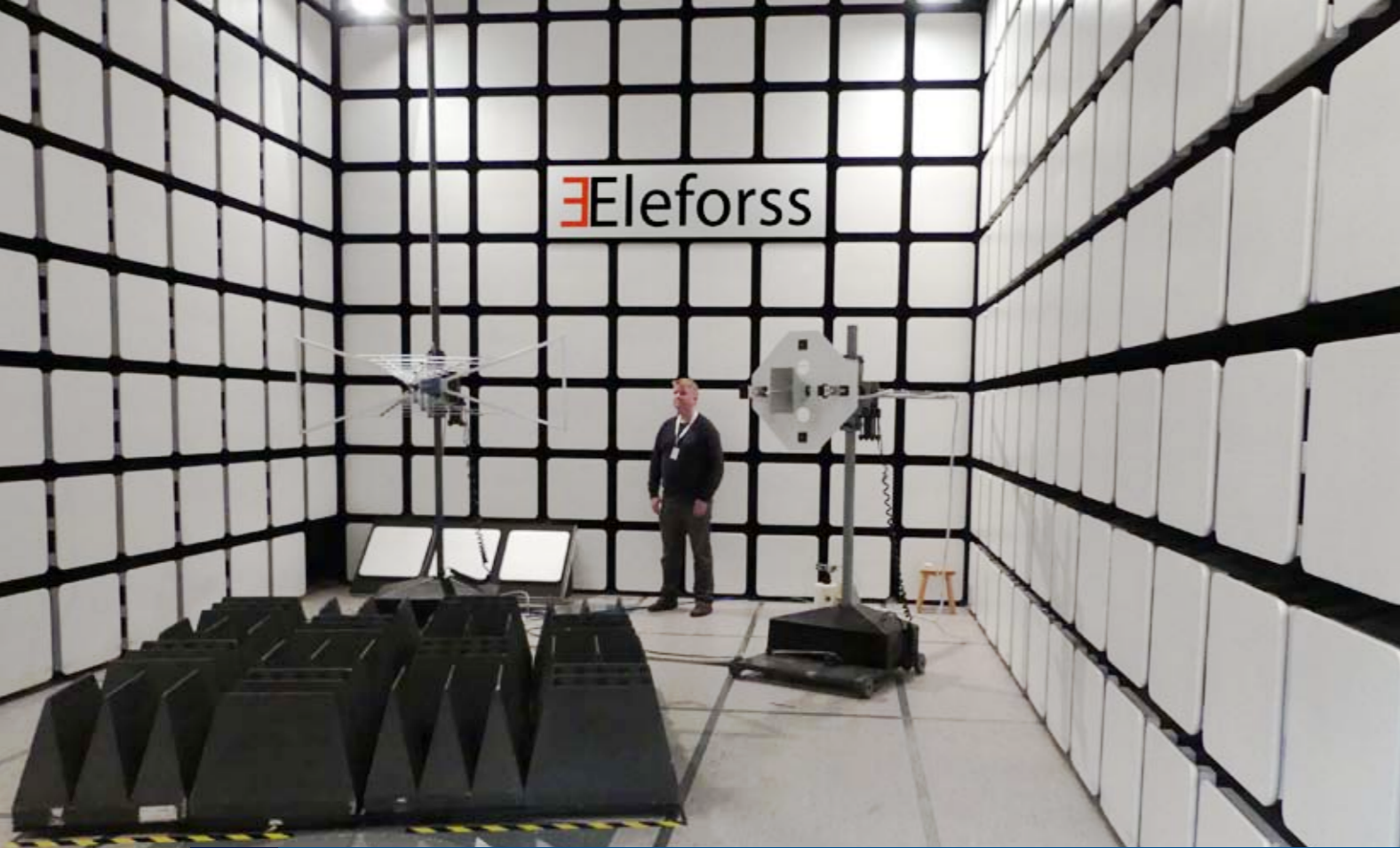
↑ Tampereen laboratoriotiloissa on mm. Full Compliance -tason Electromagnetic Compatibility (EMC) -mittaushuone.
